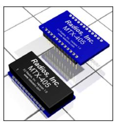
frequency dividers and a phase-detector. The output power of the power amplifier can be programmed to eight levels. A lock detect circuit detects when the PLL is in lock.
